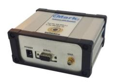
The receiver is based on an embedded platform (FPGA/DSP) and is capable of operating with lesser power consumption to allow longer duration of operations.
