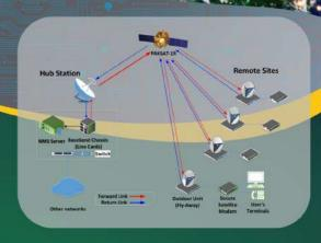
SUPARCO's Secure SatCom Network (SSN) is an indigenously developed solution for military/strategic satellite communication needs. Its goal is to provide end-to-end information security during transmission in star topology while ensuring bandwidth demands of the terminals through Multi-Frequency Adaptive Time Division Multiple Access (MF-ATDMA).
